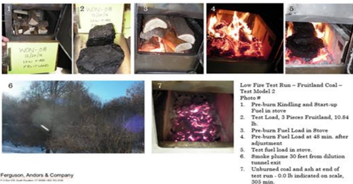
Running emissions tests on old stoves. Photo credit: Ferguson, Andors & Company
