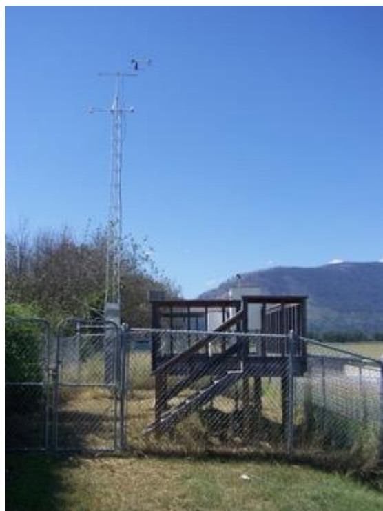
Kootenai Tribe of Idaho PM 2.5 Nephelometer and Meteorological Station
