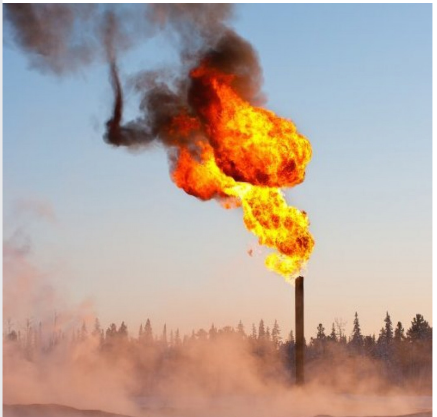
Flares burn off excess methane at an oil and gas field. Credit: Pacific Northwest National Laboratory
