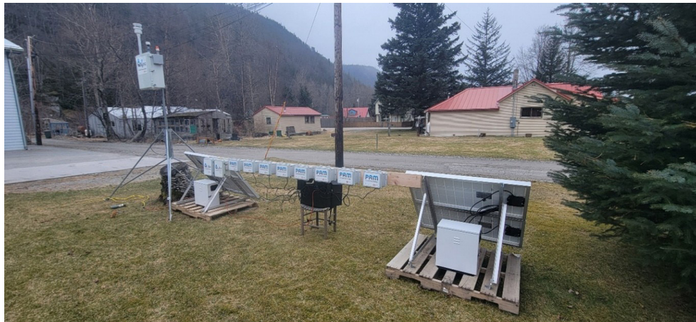
Figure 3: Collocation of 2B Technologies AQ Sync, AQ Lites, and PAMs
